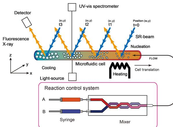
Figure 1: Schematic principle of *in-situ* XAS
