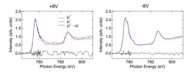
Fig.1: Depth-resolved Co L-edge XAS,  $\mu^+$  and  $\mu^-$ , and XMCD,  $\mu^+$ - $\mu^-$ , spectra of GdO<sub>x</sub>/Co thin films measured at Photon Factory BL-16A. XAS component of the interfacial Co layer is extracted. Positive (left) and negative (right) electric fields are applied to the film surface.
